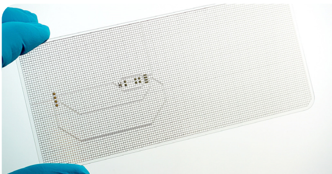
Printed semi-transparent conductors for smart window applications
