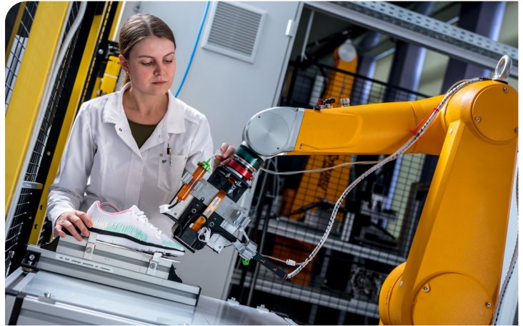
Decoration of free-form components with a robot inkjet printing system
