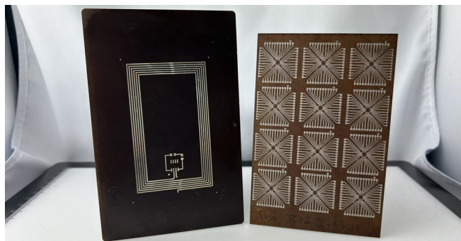
Conductive interconnections printed on sustainable lignin-based substrate
