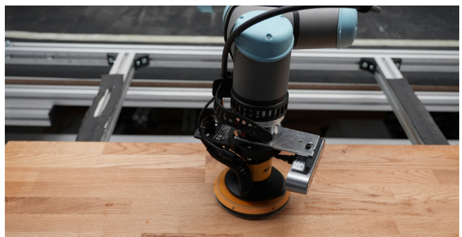
Sanding wooden panels
