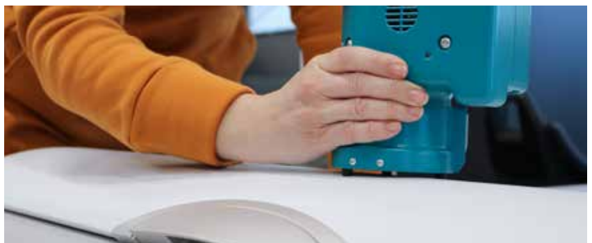
T-SCAN testing an airplane overhead compartment
